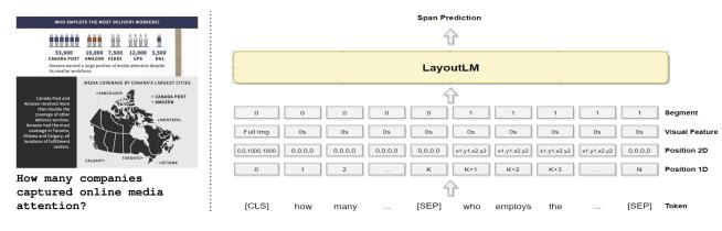
Figure 5: Overview of our LayoutLM based model for predicting answer spans. Textual, visual and layout modalities are embedded and mapped to the same space. Then, they are added and passed as input to a stack of Transformer layers.
